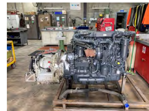
Scania engine rebuilt with ZF gearbox attached
