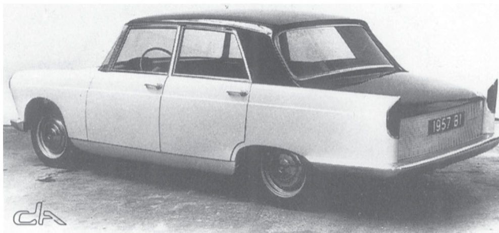
The first full-size mock-up submitted by Pinin in 1957. On the rear, the low part in aluminium wasn't appreciated by Peugeot management who asked to delete it.
