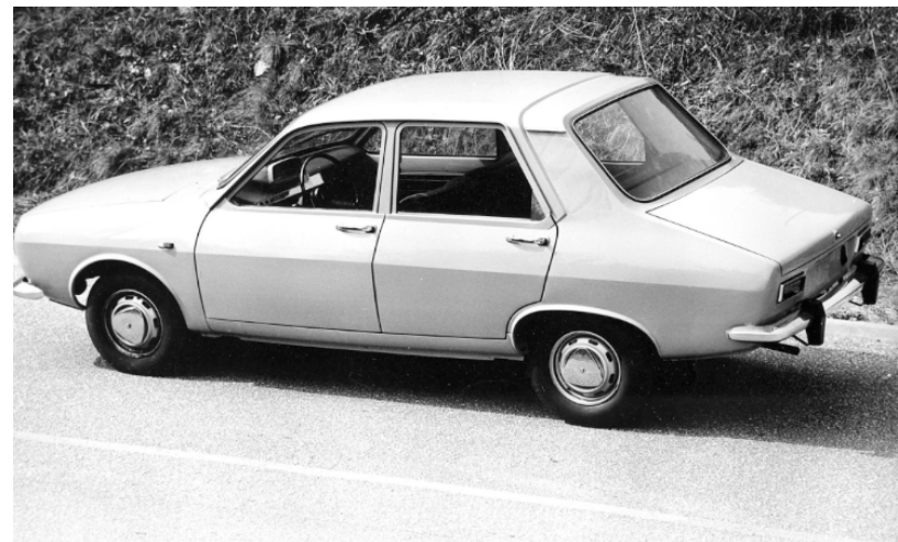
One of the first prototypes of the Renault 12 with specific hubcaps, closer rear lights and a gutter on the C-pillar.
